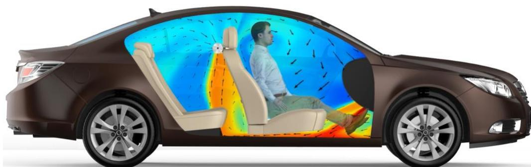
*Figure 1: Air flow inside a car cabin when using the Airbubbl. Blue/light blue indicates clean air, while red/orange/green indicates polluted air.*
